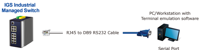
Figure 4-1: Industrial L2+ Managed Switch Console Connectivity
